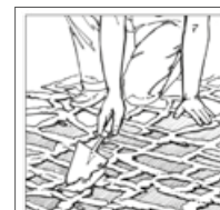
Sgrossata Removing Excessive Grout
