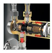
Effective protection against scalding: If the cold water cuts out, the hot water inlet is closed immediately.
