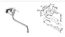
KLUDI LOGO NEO single lever bath- and shower mixer DN 15 solid lever wall fastening distance from center to center 45 mm flow class BA aerator M 22 x 1/B ceramic cartridge with hot water limitation swivelling spout 250 mm s-connections G 1/2 x G 1/2 protected against back flow noise-level II PA-IX 3967/IIBA
