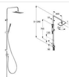
**KLUDI A-QA Dual-Shower-System DN 15** wall fastening with horizontally and vertically adjustable tube flow class AA two-way ceramic diverter water supply with flexible hose G 1/2 x G 1/2 x 800 mm horizontal and vertical adjustable slider KLUDI SUPARAFLEX SILVER G 1/2 x G 1/2 x 1600 mm with KLUDI A-QA headshower G 1/2 x 140 x 245 mm with KLUDI A-QA hand shower with one spray mode with mounting material
