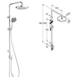
KLUDI A-QA Dual-Shower-System DN 15 with horizontally and vertically adjustable tube wall fastening wall fastening two-way ceramic diverter water supply with flexible hose G 1/2 x G 1/2 x 800 mm with horizontal and vertical adjustable slider KLUDI SUPARAFLEX Hose DN 15 G 1/2 x G 1/2 x 1600 mm with KLUDI A-QA headshower Ø 250 mm, swiveling KLUDI A-QA s hand shower DN 15 with three spray patterns with mounting material without shower mixer
