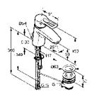
KLUDI MX single lever basin mixer DN 10 open ring lever single hole mounted flow class A s-pointer aerator M 24 x 1 ceramic cartridge with hot water limitation pop-up waste G 1 1/4 flexible hoses G 3/8 rapid installation set
