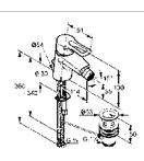
KLUDI MX single lever bidet mixer DN 10 open ring lever single hole mounted flow class Z ball joint-cascade-aerator M 24 x 1 ceramic cartridge with hot water limitation pop-up waste G 1 1/4 flexible hoses G 3/8 rapid installation set
