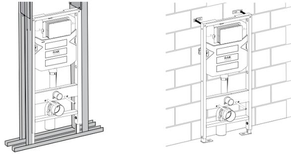
With a drywall system it is possible to create complete room-height prewalls or partitions.
