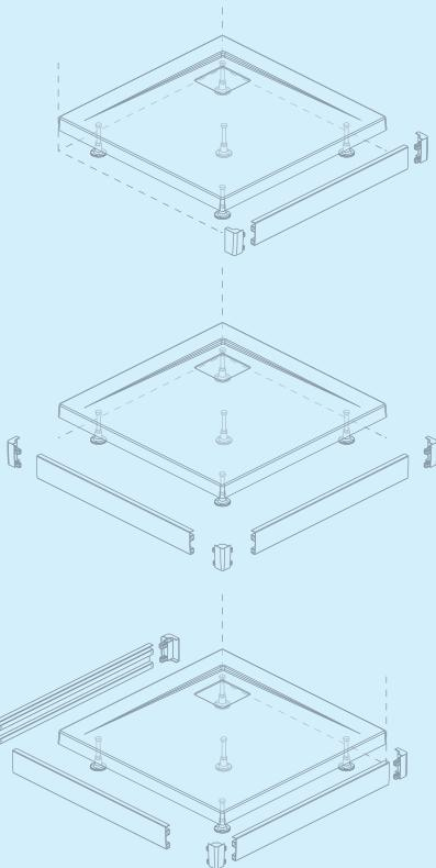
**Front panel** (for recess doors) – a shower tray with legs, 1 panel, 2 endings in appropriate finish colour
